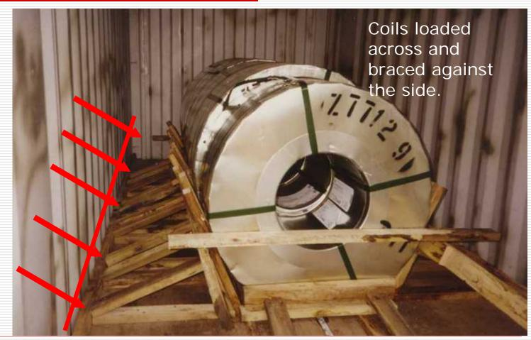
Note the longitudinal layers stretching the pressure along the wall
