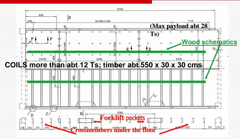
Always min. 2x layers in the width and never any coil touching the floor.
