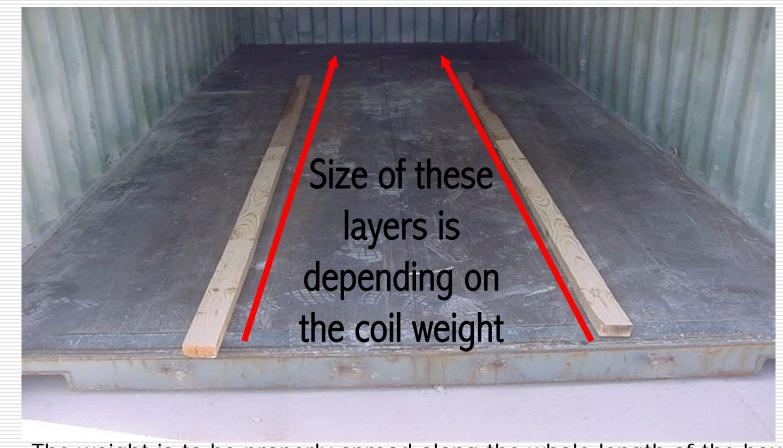
The weight is to be properly spread along the whole length of the box.
